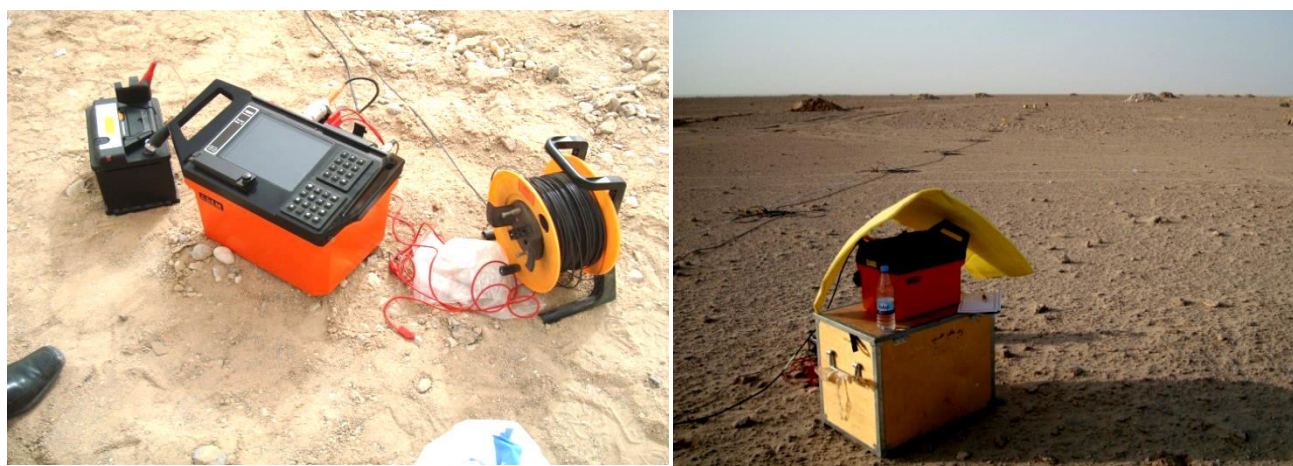
Figure (28) : The modern instrument of seismic refraction – refraction surveying.
