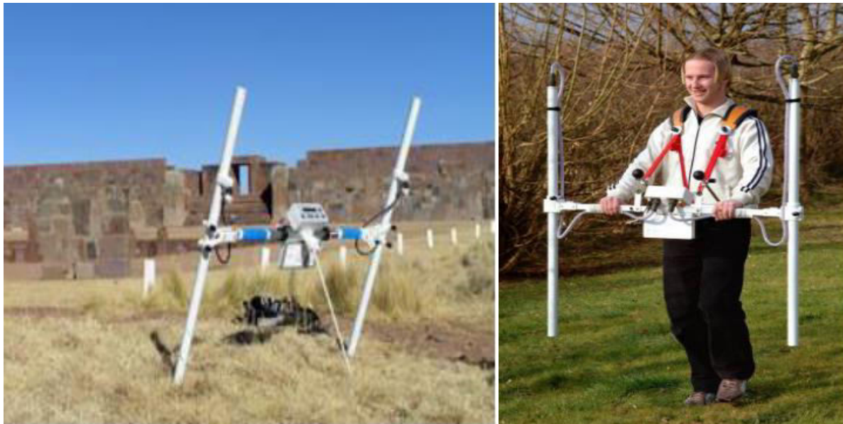
Figure (20): The magnetic gradiometer in use during field surveying.
