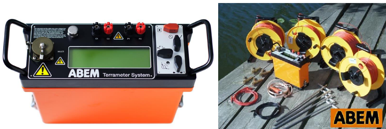
Figure (5): The ABEM 1000 Terrameter system which used in the 1D resistivity survey.
