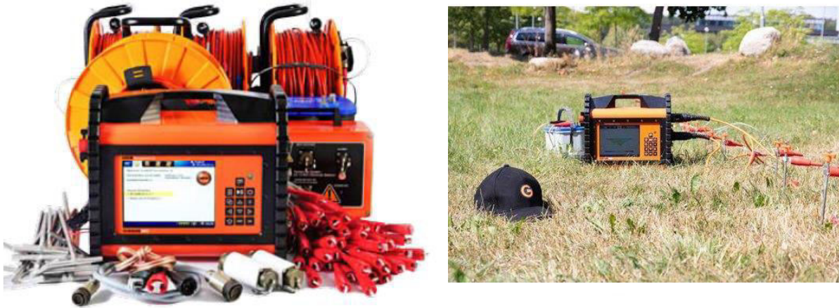
Figure (6): The ABEM Terrameter LS system which used in the 2D and 3D electrical resistivity tomography surveys.
